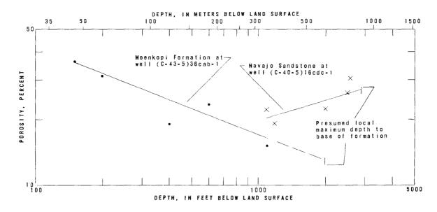
Figure 7.— Relation between porosity and depth for two aquifers in the upper Kanab Creek basin.
