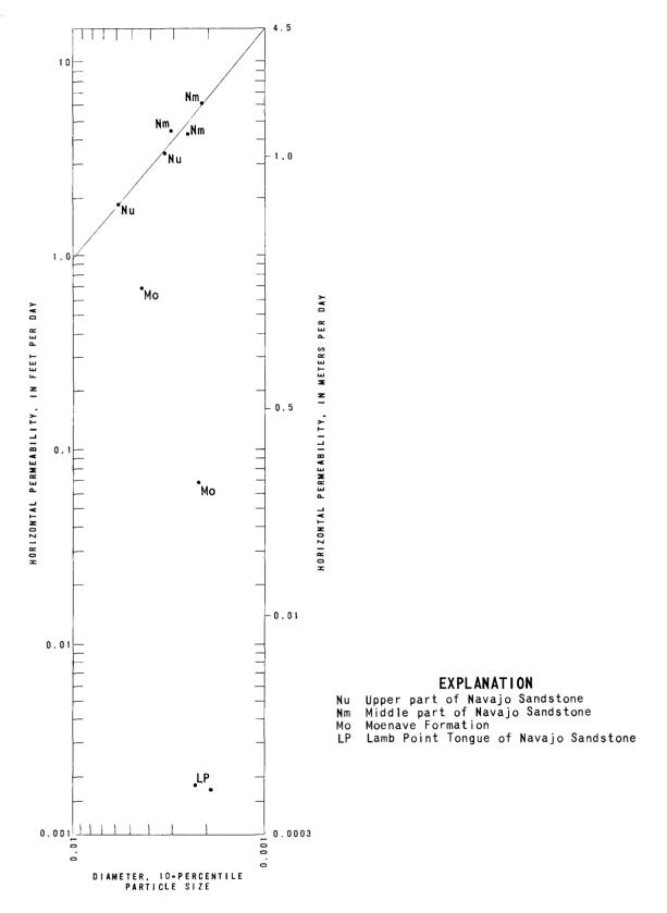
Figure 8. - Relation of horizontal permeability to the IO-percentile particle-size diameter of selected rock samples.
