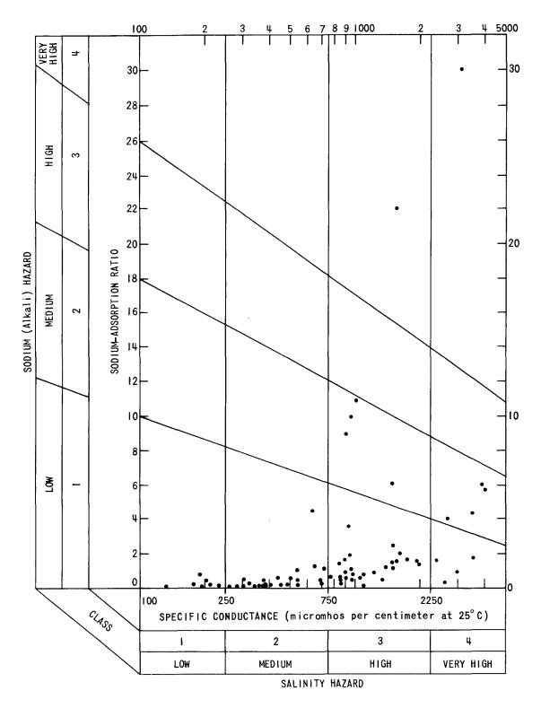
Figure 15.— Classification for irrigation of selected ground-water samples from the study area. (Classification after a method of the U.S. Salinity Laboratory Staff, 1954.)
