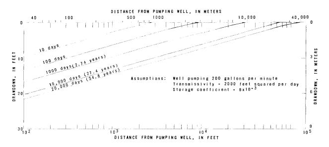
Figure 18. — Theoretical relation between drawdown and distance from a pumping well tapping mainly the Shinarump Member of the Chinle Formation for selected pumping durations.
