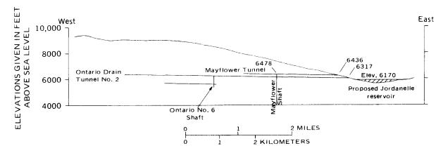
Figure 12.– Generalized section showing relationship of the proposed Jordanelle reservoir to the Mayflower Tunnel and shaft, the Ontario No. 2 Tunnel, and the Ontario No. 6 shaft. (Modified from UINTEX CORP., 1984, fig. 2).
