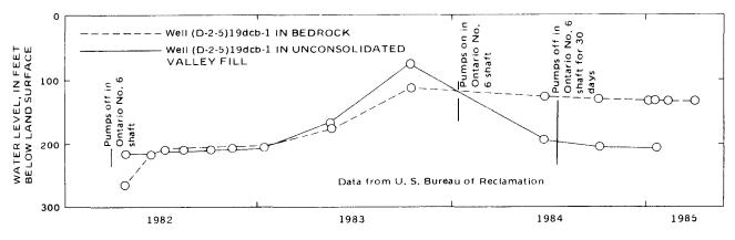
Figure 11.—Relationship of water levels in wells (D-2-5)19dcb-1 and (D-2-5)19dcb-2 to dewatering operations in the Ontario No. 6 Shaft.
