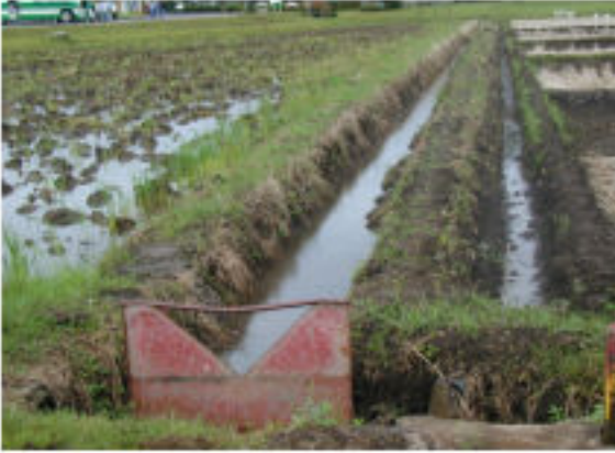
Figure 2: V-Notch Weir in the Field
