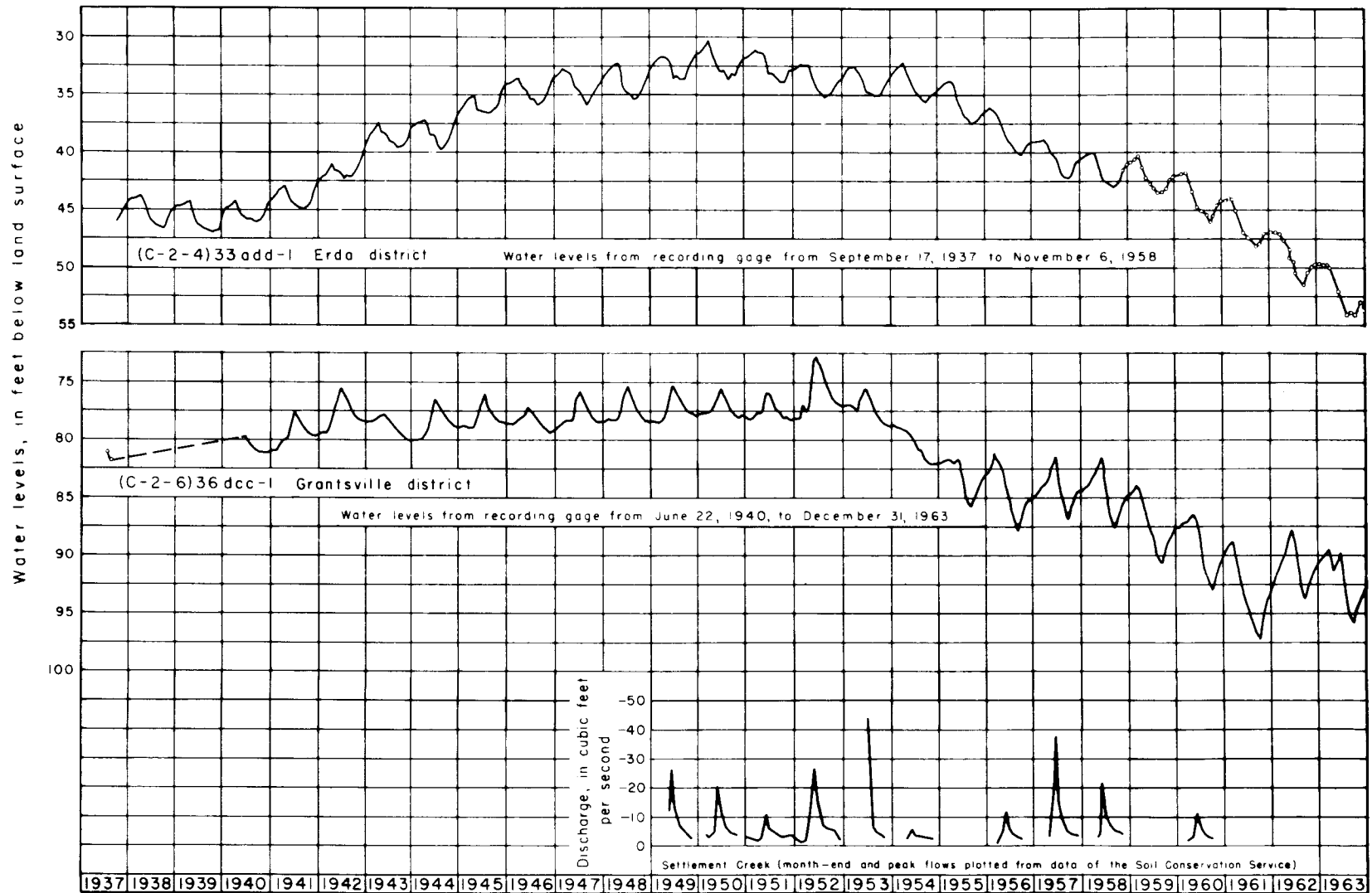
Figure 7.—Hydrographs of two wells in Tooele Valley, 1937-63, and discharge of Settlement Creek 1949-60.
