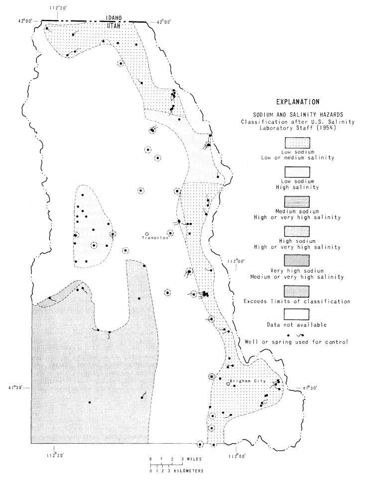
Figure 8.- Areal distribution of sodium and salinity hazards of water from the principal ground-water system.
