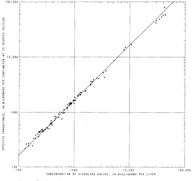
Figure 7.--Relation of specific conductance to the concentration of dissolved solids in ground water in the lower Bear River drainage basin.
