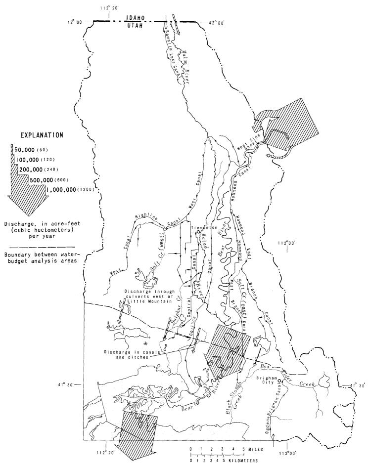
Figure 3.- Flow diagram showing streams, canals, and average annual discharge of principal streams crossing boundaries of water-budget analysis areas, water years 1960-71.
