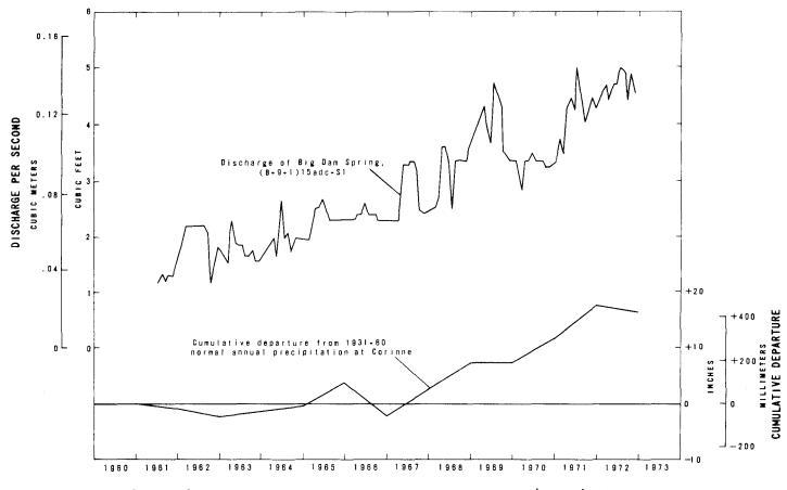
Figure 6.- Relation of discharge of Big Dam Spring, (B-9-1)|5adc-SI, to cumulative departure from the 1931-60 normal annual precipitation at Corinne.
