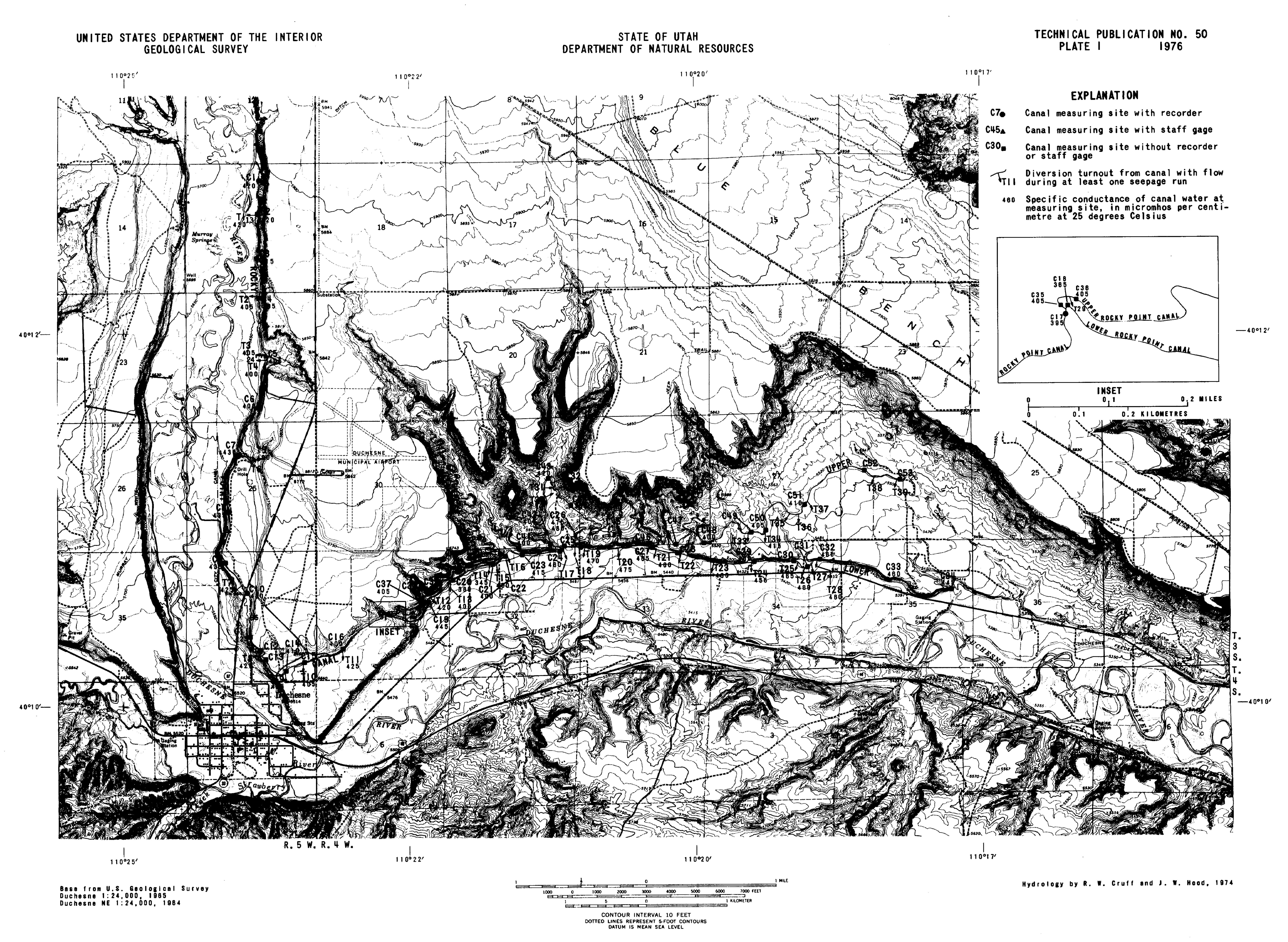
MAP SHOWING LOCATIONS OF CANAL AND OTHER MEASUREMENT SITES AND SPECIFIC CONDUCTANCE OF WATER DURING SEEPAGE MEASUREMENTS, AUGUST 30, 1972, ROCKY POINT CANAL SYSTEM, DUCHESNE COUNTY, UTAH
