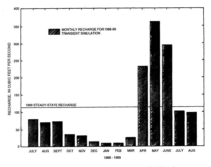
Figure 22.--Monthly recharge for the 1988-89 transient simulation and 1989 steady-state recharge.
