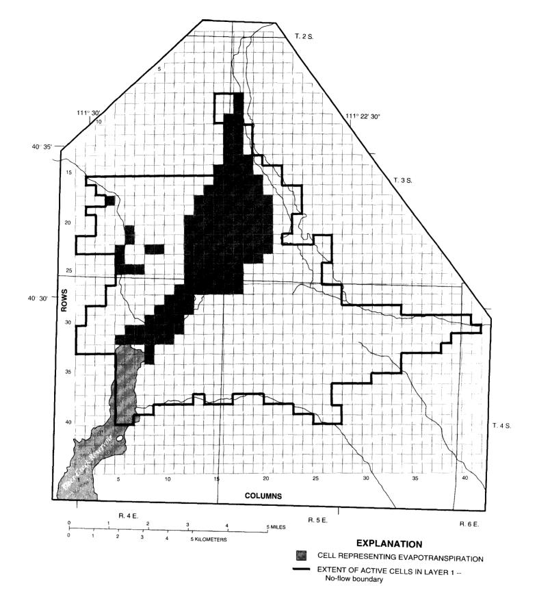
Figure 17.--Location of cells used to simulate evapotranspiration.
