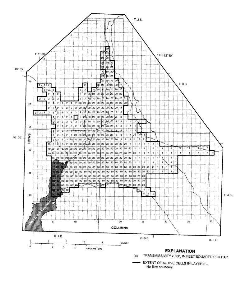
Figure 14.--Distribution of transmissivity in layer 2.
