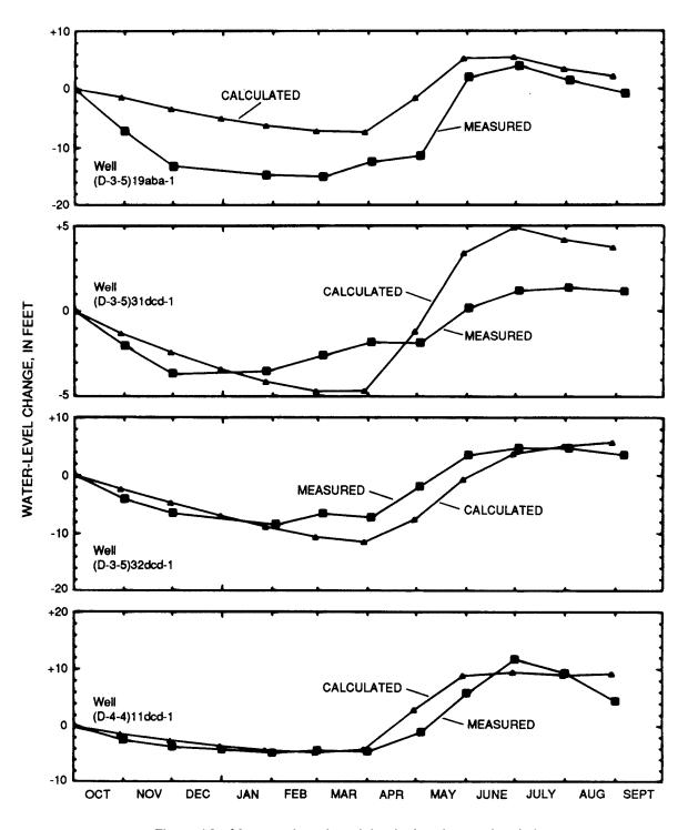
Figure 20.--Measured and model-calculated water-level changes for the 1949-50 monthly transient-state simulation.
