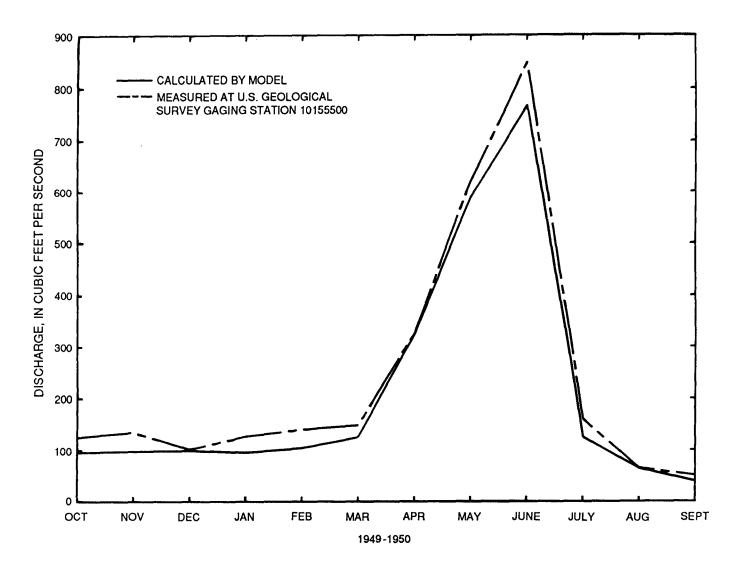
Figure 21.--Measured discharge at U.S. Geological Survey gaging station 10155500 from October 1949 to September 1950 and model-calculated discharge of the Provo River.
