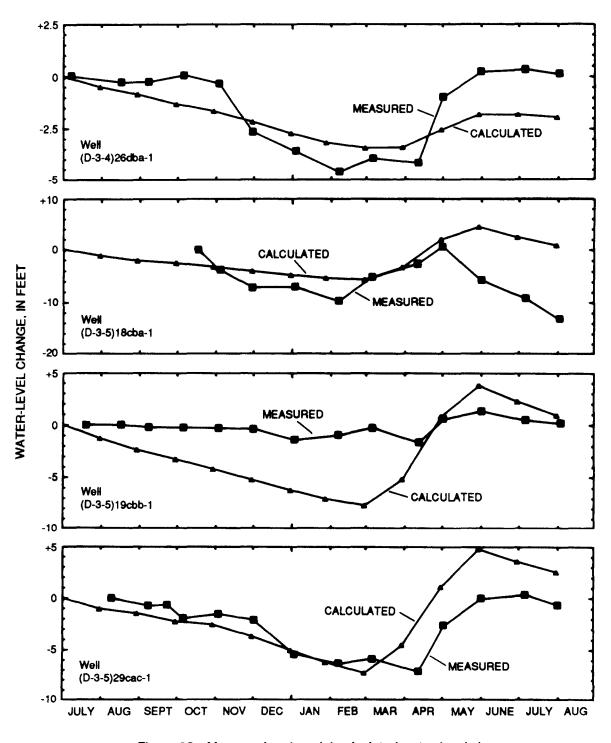
Figure 23.--Measured and model-calculated water-level changes for the 1988-89 monthly transient-state simulation.
