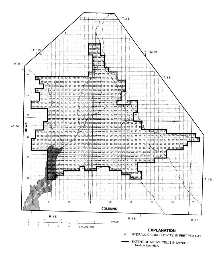
Figure 13.--Distribution of hydraulic conductivity in layer 1.
