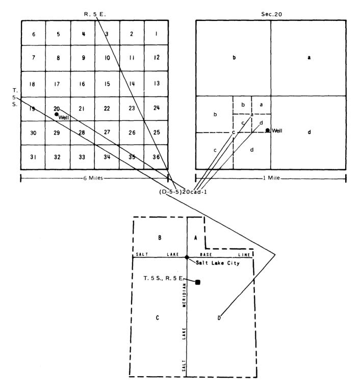
Figure 2.--Numbering system for hydrologic-data sites.
