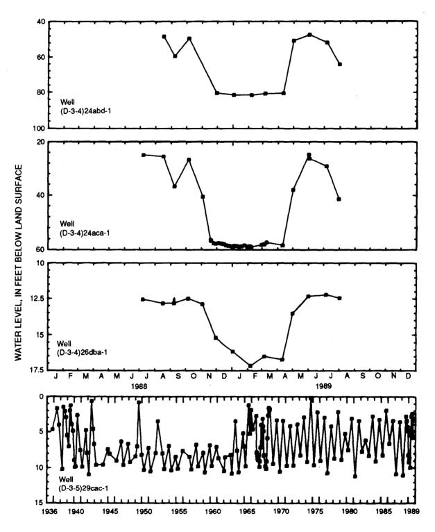
Figure 5.--Water levels in selected wells completed in unconsolidated valley-fill deposits.
