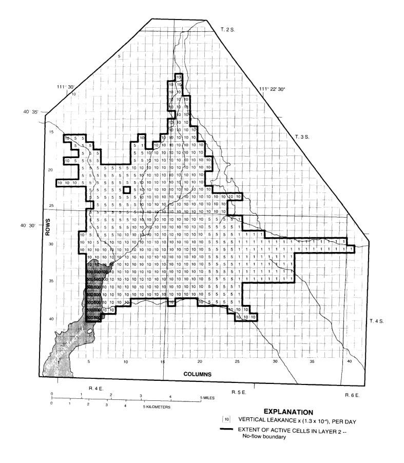
Figure 15.--Distribution of vertical leakance between layers 1 and 2.
