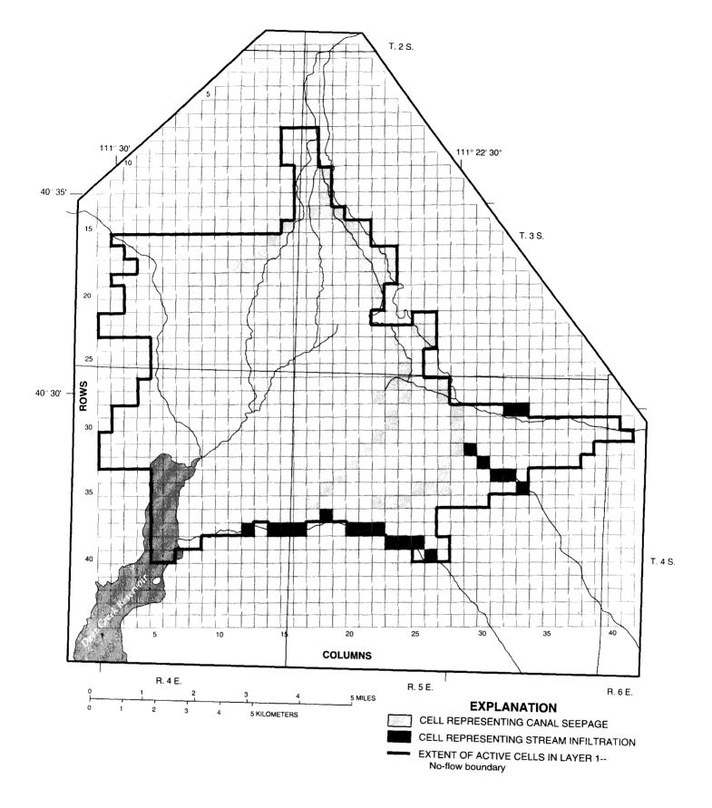
Figure 11.--Location of cells used to simulate recharge from canal seepage and stream infiltration.
