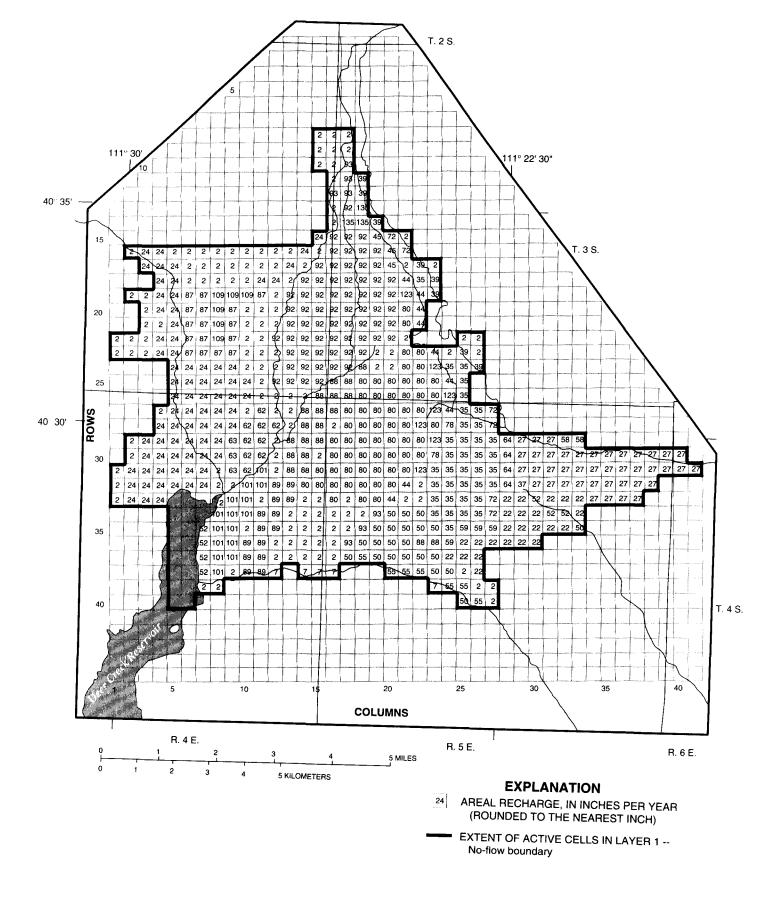
Figure 12.--Distribution of areal recharge used in the 1950 steady-state simulation.
