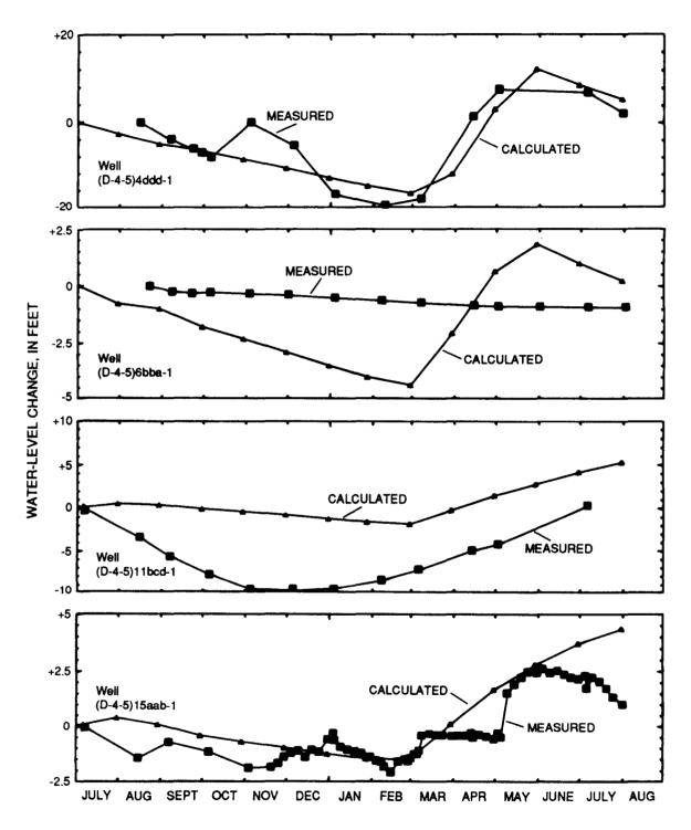
Figure 23.--Measured and model-calculated water-level changes for the 1988-89 monthly transient-state simulation--Continued.
