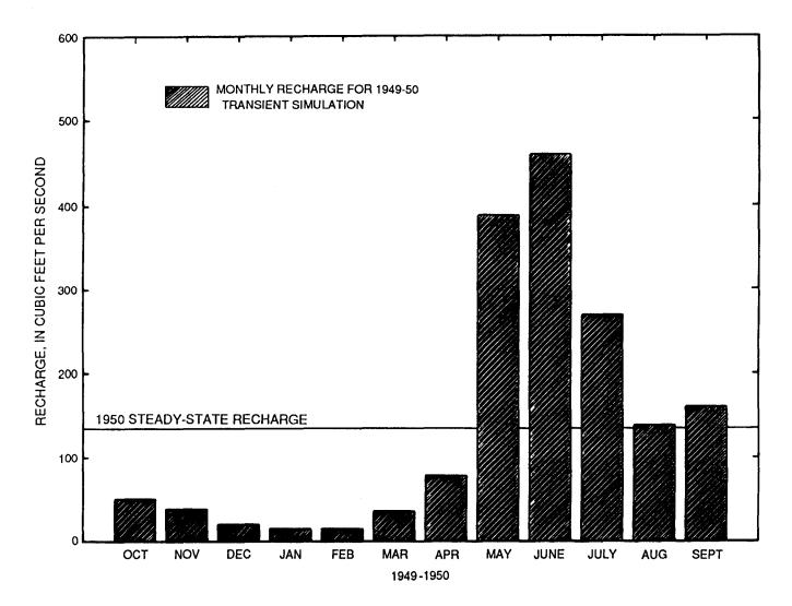
Figure 19.--Monthly recharge for the 1949-50 transient simulation and 1950 steady-state recharge.
