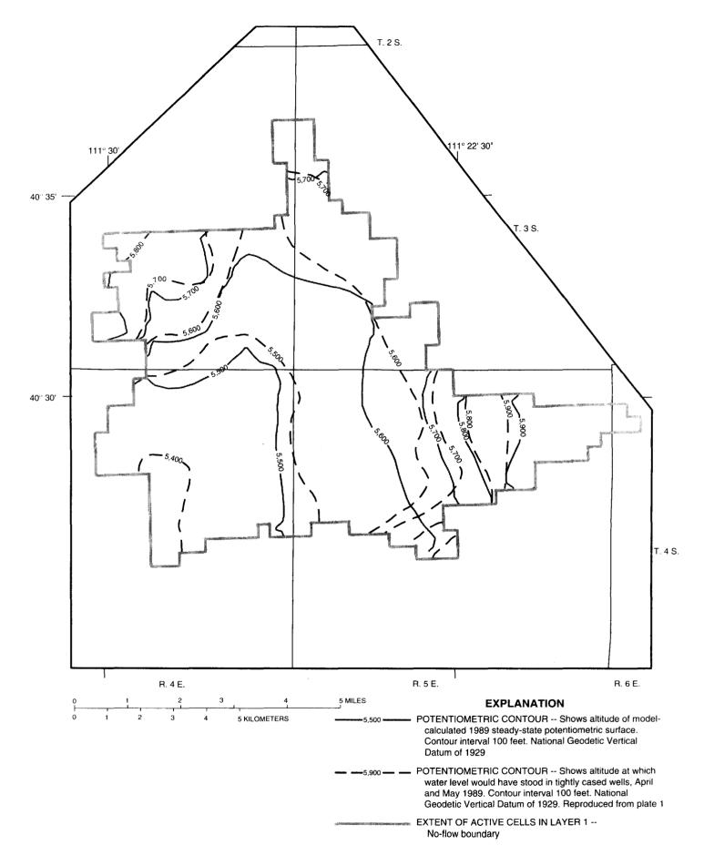
Figure 24.--Potentiometric surface in April and May of 1989 and simulated 1989 steady-state potentiometric surface.
