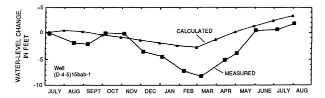
Figure 23.--Measured and model-calculated water-level changes for the 1988-89 monthly transient-state simulation--Continued.
