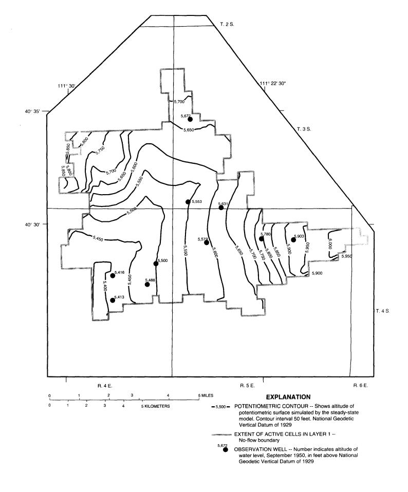
Figure 18.--Altitude of water levels in observation wells, September 1950, and simulated 1950 steady-state potentiometric surface.
