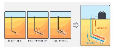
surface. Once through the plant, the spent water is recirculated back into the injection well and the process repeats.
