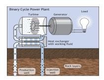
surface, or hot groundwater flashing a working fluid in a binary cycle system. Spent geothermal fluids are then injected back into the geothermal reservoir from which they came. Power production from hot groundwater (steam or brine) is considered a beneficial use, and a water right is required for this type of system.
