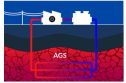
electricity through a modular binary cycle turbine generator plant. The spent working fluid is then reinjected and continues to recirculate through the system.
